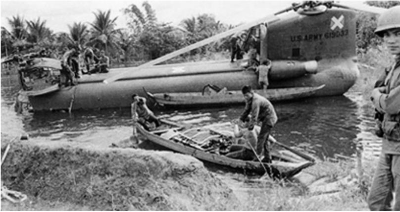
gines were then rigged to be sling loaded off the downed aircraft. Machen and Parker then took the recovery aircraft and hovered over the downed aircraft. With precise guidance from Ray Todorovich, each of the engines were removed, loaded into a waiting boat and later, without damage to the engines, loaded aboard the recovery aircraft. Before nightfall, all the equipment above the water level inside the downed aircraft was removed.
